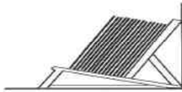
Incorrect method of stacking
